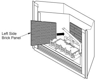
Figure 39 - Installing Brick Panels
